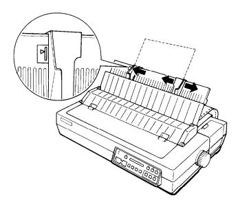
5. Slide **a** sheet of paper down between the edge guides until it meets resistance.
